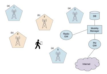
The user device is registered with operator (a), and gets the following beacons from the different towers with different received signal strength indicators (RSSI).
