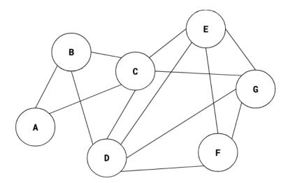
The diagram above shows a L2 network where all links have equal cost. We want to apply the Spanning Tree Protocol. Choose the switch with the lowest alphabetical ID as the root, and when there are multiple shortest paths to the root, choose the path that uses the neighbor switch with the lowest alphabetical ID.
