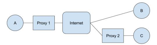
Consider the (abstracted) network topology above. Hosts A and C are connected to HTTP proxies that cache the results of the last two HTTP requests they've seen to improve performance. The proxy will perform any TCP handshakes or teardowns with the client and server concurrently. That is, when it gets a SYN from a client, it will respond and immediately send a SYN to the server, and similarly for other messages.
